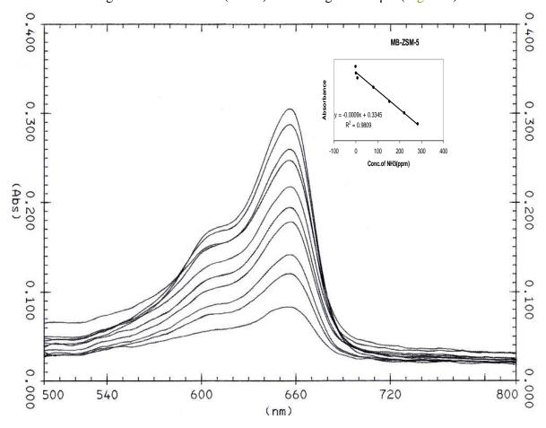
Fig.1. UV-vis spectra of the reduction of MB by varing amounts of ammonia in nanomordenite zeolite . Inset shows the absorbance vs. concentration of ammonia (ppm) plot
