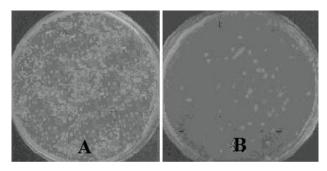
Fig.6.S.dysenteriae growing on the agar medium without ZnO nanoparticles (A) and with 1% nano-ZnO (B)
