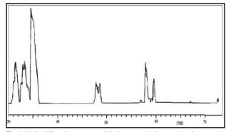
Fig.1.XRD diffraction spectra of ZnO nanoparticles powder for sample  $2hr-160^{\circ}C-2-180^{\circ}C$ .
