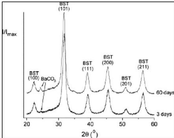
Fig.11. X-ray diffractogram of the Ba<sub>0.8</sub>Sr<sub>0.2</sub>TiO<sub>3</sub> powder collected 3 days and 60 days after synthesis [63].
