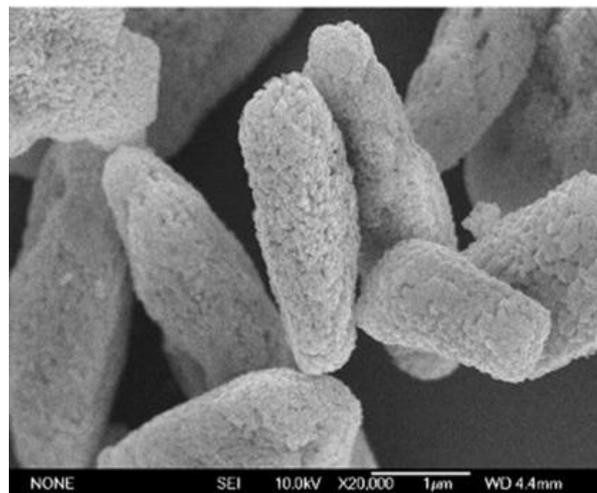
Fig.9. SEM images of surface of BST powders, with PEG [14]
