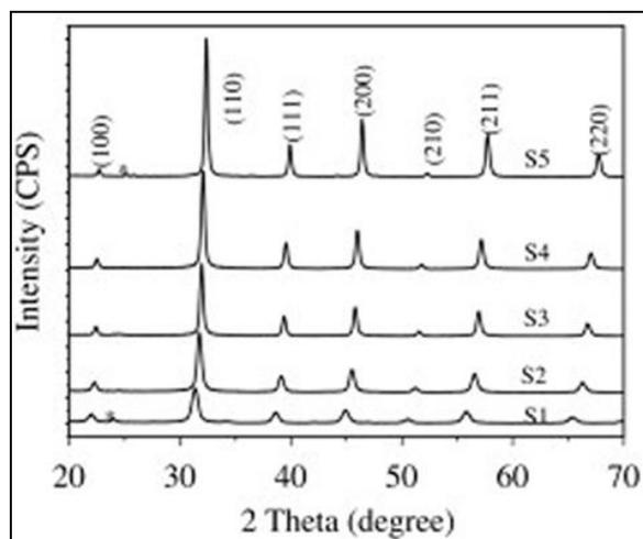
**Fig.10.** XRD patterns of the as-synthesized BST nanocrystal powders in the  $2\theta$  range of  $20^\circ$ – $70^\circ$ . The asterisks marked in the figure represent the tiny by-products of carbonate [7].
