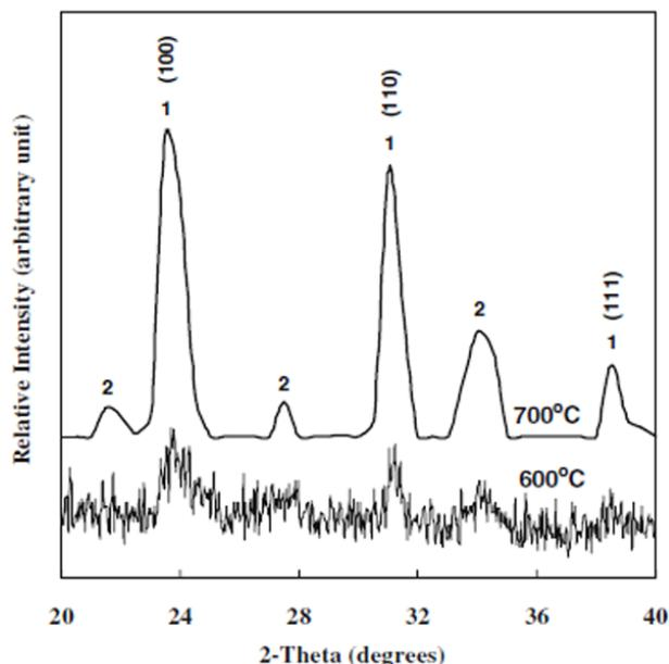
Fig.23. XRD patterns of BST nanopowder calcined at 600 and 700°C, separately, for 2 h.  $\text{Ba}_{0.7}\text{Sr}_{0.3}\text{TiO}_3$  and  $\text{Ba}_4\text{Ti}_3\text{O}_{30}$  peaks, observed in these XRD traces, are marked as 1 and 2, respectively [68].
