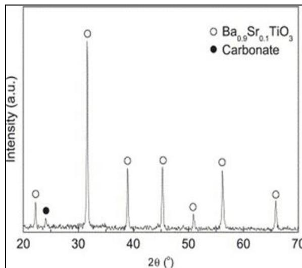
Fig.2. X-ray diffraction pattern of (Ba<sub>0.9</sub>Sr<sub>0.1</sub>)TiO<sub>3</sub> nano-particles [13].
