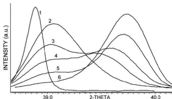
**Fig.19.** (1 1 1) peak of Ba-pure (1) and five samples prepared with different Ba:Sr mol ratios of 0.9:0.1 (2), 0.85:0.15 (3), 0.8:0.2 (4), 0.75:0.25 (5), and 0.7:0.3 (6). The experimental curves were smoothed for a better view [45].
