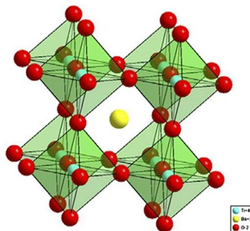
Fig.1.Perovskite structure [47].
