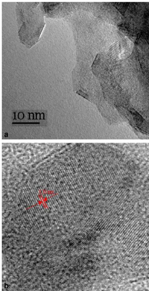
**Fig.24.** (a) TEM micrograph of BST powder calcined at 700°C. (b) TEM micrographs showing lattice fringes and interplanar distance (0.38 nm) of Ba<sub>0.7</sub>Sr<sub>0.3</sub>TiO<sub>3</sub> phase [68].
