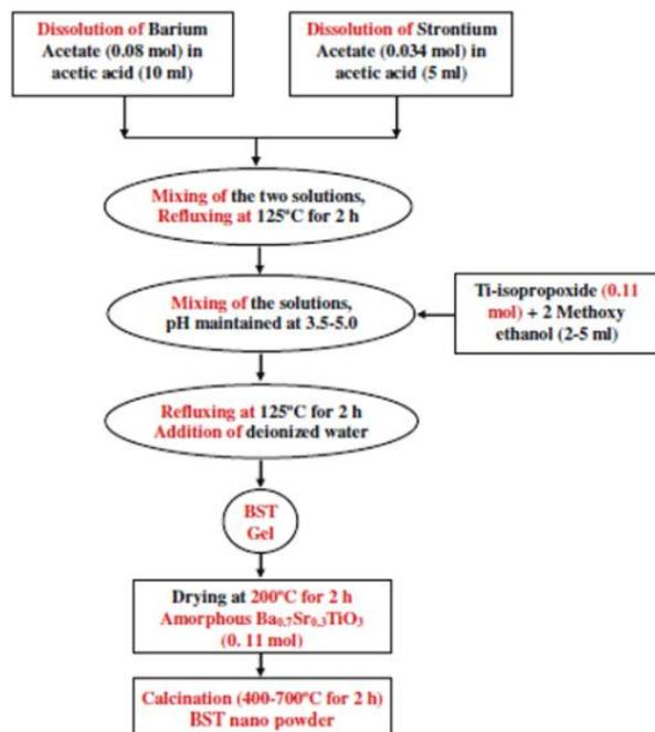
Fig.22. Schematic detailing synthesis of nanocrystalline BST powder [68]
