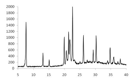
Fig.2. XRD pattern of the prepared AlPO<sub>4</sub>-5 crystals
