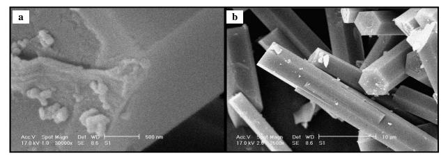
Fig.3. SEM image of the prepared AlPO<sub>4</sub>-5 crystals; (a) 30000 X and (b) 2500 X
