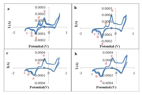
Fig. 1. Voltammograms of Fe-doped MWCNTS at scan rates of (a) 20, (b) 50, (c) 100 and (d) 200 mVs<sup>-1</sup>.
