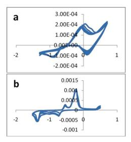
Fig. 3. Cyclic voltammogram of the (a) bare electrode (b) Ni electrodeposited electrode via CV method at scan rate of  $50~mVs^{-1}$
