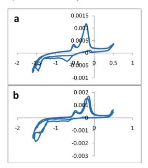
Fig. 4. Cyclic voltammogram of Ni electrodeposited electrode via duble-pulse technique at scan rate of 20 mV  $\rm s^{\text{-}1}$
