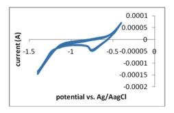
Fig. 2. Cylic voltammogram of electrodeposition of Ni nanoparticles on electrode at scan rate of 50 mV s  $^{\text{-1}}$
