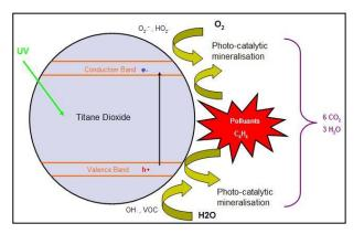
Fig.1. Photocatalysis on anatase TiO<sub>2</sub>
