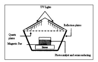
Fig. 2. Photocatalysis Reactor
