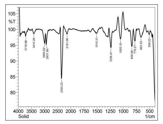
Fig. 14. FTIR spectra of TiO<sub>2</sub> on Methylene blue after photodegradation
