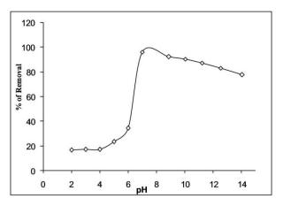
Fig. 3. Effect of pH on adsorption of Methylene blue on  $\mathrm{TiO}_2$
