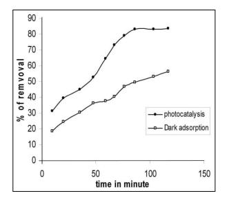
Fig. 16. Photocatalysis and dark adsorption of Methylene blue
