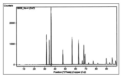
Fig.8. XRD diagram of ZnO semiconductor after irradiation
