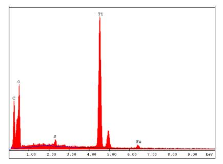
Fig. 11. EDX pattern of TiO<sub>2</sub>
