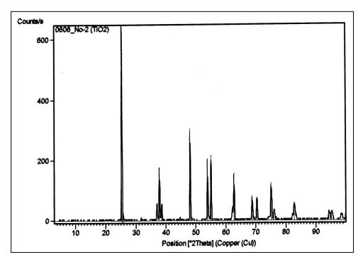
Fig. 7. XRD diagram of TiO<sub>2</sub> semiconductor after irradiation
