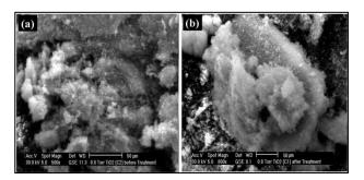
Fig. 9. SEM images of TiO2 a) before treatment b) after treatment
