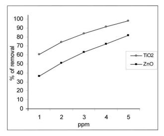
Fig.6. Effect of Photocatalyst dose
