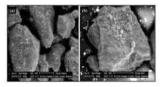
Fig.10. SEM images of ZnO  $\,$  c) before treatment d) after treatment
