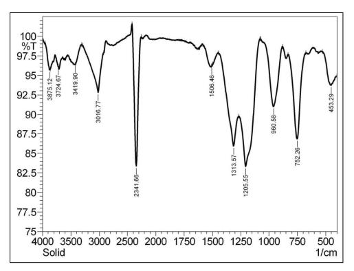
Fig. 13. FTIR spectra of  $TiO_2$  on Methylene blue before photodegradation  $TiO_2$
