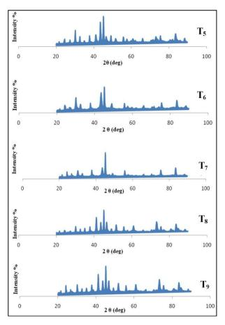
**Fig. 2.** The XRD patterns of samples synthesized powder using thiourea fuel ( $T_5$ ,  $T_6$ ,  $T_7$ ,  $T_8$  and  $T_9$ ) at different pH from5 to 9.
