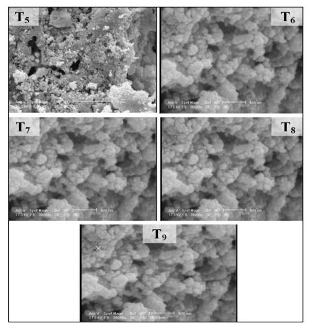
**Fig. 4.** The SEM images for all samples prepared with thiourea fuel  $(T_5, T_6, T_7, T_8 \text{ and } T_9)$  at different pH from 5 to 9.
