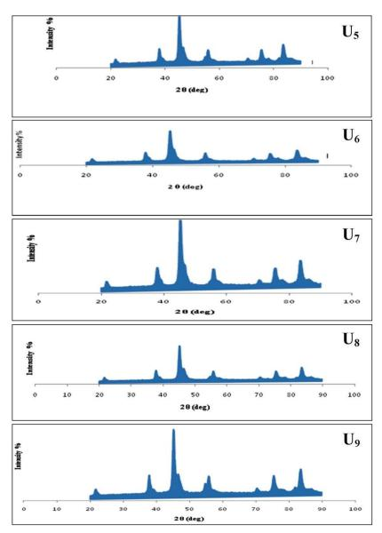
Fig. 1. The XRD patterns of the as-synthesized powder urea route (U<sub>5</sub>, U<sub>6</sub>, U<sub>7</sub>, U<sub>8</sub> and U<sub>9</sub>) at different pH from 5 to 9.
