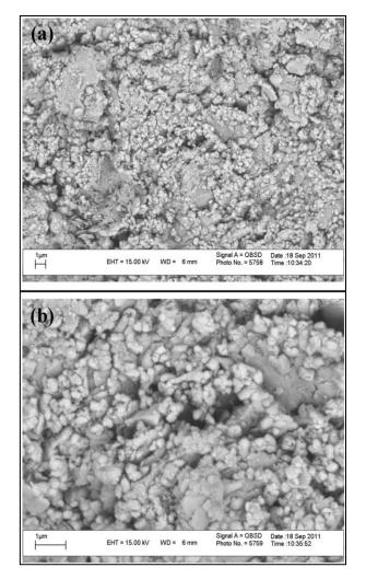
Fig. 3. Microstructure of normal concrete at different scale
