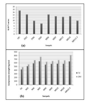
Fig. 2. Test results graphs (a) The permeability index (b) Compressive strength of 7,28 days
