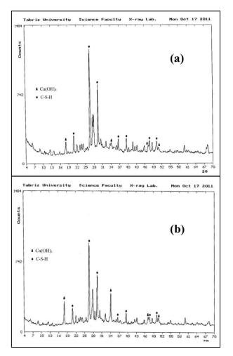
Fig. 5. XRD results of concrete at the curing age of 28 days (A) concrete with nano-silica (B) normal concrete
