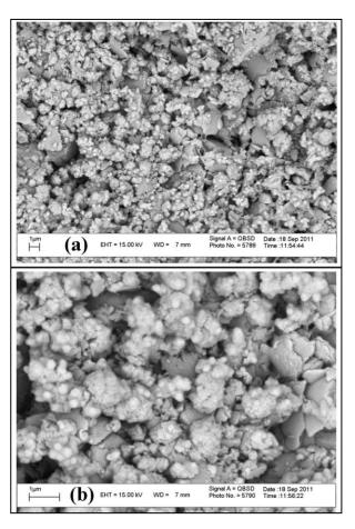
Fig. 4. Microstructure of Nano-Silica concrete at different scale
