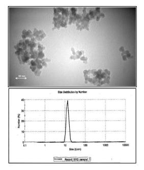
Fig. 1. TEM of nano- SiO2 and size distribution diagrams of SiO2 nano particles
