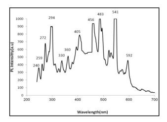
Fig. 6. PL spectrum from nanoCaF $_2$ ,  $\lambda ex=218nm$
