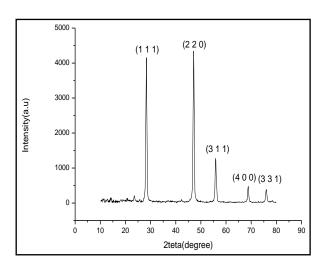
Fig. 2. XRD plot of an undoped sample of nano CaF<sub>2</sub>
