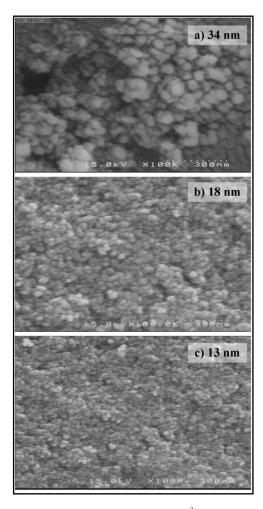
Fug. 9 SME picture of a) nano  $CaF_2$  b)  $CaF_2$ : $Ce^{3+}$  nanoprticles 5% c)  $CaF_2$ : $Ce^{3+}$  nanoprticles 10% (with average size of them)
