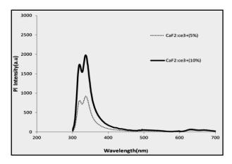
**Fig. 7.** PL spectrum from CaF<sub>2</sub>: Ce<sup>3+</sup> nanoparticles with different dopping percent
