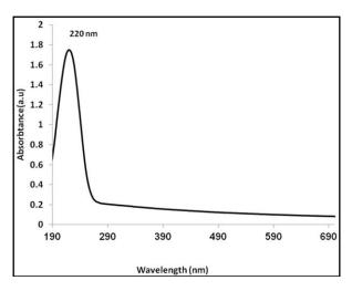
Fig. 4. Optical absorption spectrum of nano CaF<sub>2</sub>
