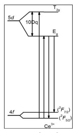
Fig. 8. Schematic levels of Ce<sup>3+</sup> in CaF<sub>2</sub>:Ce<sup>3+</sup> nanoparticles
