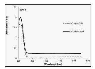
**Fig. 5.** Optical absorption spectrum of CaF<sub>2</sub>: Ce<sup>3+</sup> nanoparticles with different dopping percent
