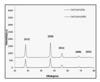
**Fig. 3.** Comparison between XRD plot of CaF<sub>2</sub>:Ce<sup>3+</sup> nanoparticles with different dopping percent
