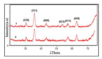
Fig. 1. Effect of concentration of ammonia on the diffraction pattern.
