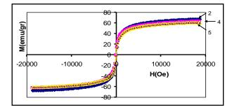
**Fig. 3.** The effect of reaction temperature on the hystersis curves of nanoparticles
