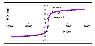
**Fig. 4.** The effect of concentration of ammonia on the hystersis curves of nanoparticles
