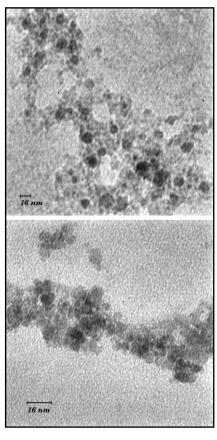
**Fig. 6.** TEM image of sample 1; reaction temperature: 90°C and concentration of ammonia: 0.5 mol/L (Left) and TEM image of sample 4; reaction temperature: 60°C and concentration of ammonia: 3 mol/L (Right)
