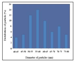
Fig. 5. The histogram of CdO nanoparticles
