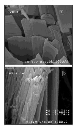
Fig. 1. SEM images of compound 1nano-structure.
