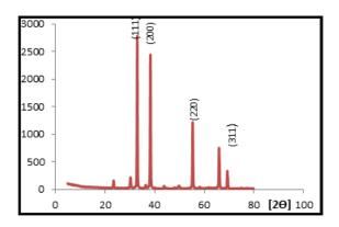
Fig. 3. XRD pattern of the prepared CdO nanoparticles
