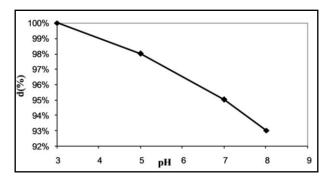
**Fig. 7.** Effect of pH on the degradation of RR222, [dye]<sub>o</sub>=20ppm and H=20
