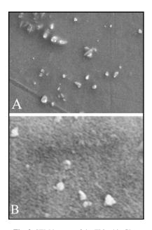
Fig. 3. SEM images of the TiO<sub>2</sub> thin film (A) 1 cycle coating without using PEG, (B) 3 cycle coating with using 0.3 gr PEG 10%.
