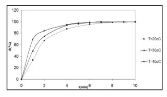
**Fig. 8.** Effect of temperature on the degradation of RR222, pH=3, [dye]<sub>o</sub>=20ppm and H=20
