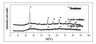
Fig. 2. XRD patterns of 1 and 3 cycles coating of TiO<sub>2</sub> films
