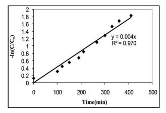
Fig. 10. The kinetic data for photocatalytic degradation of RR222 in the presence of  $TiO_2$  thin film
