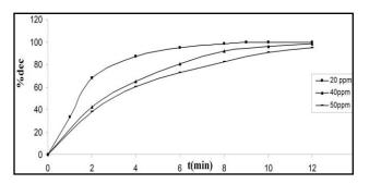
Fig. 9. Photocatalytic degradation of RR222 at different initial dye concentration, pH=3, T=20°C and H=20
