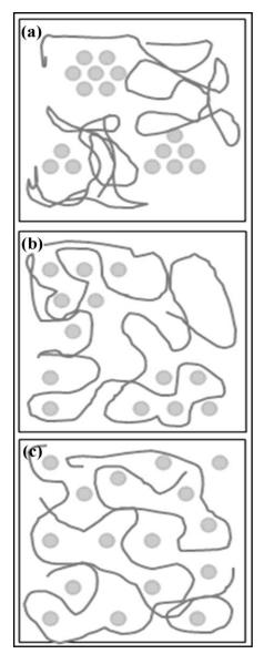
Fig. 2. Scheme of different types of nano-composites: 1.A) phase separated nano-composite, 1.B) intercalated nano-composite and 1.C) exfoliated nano-composite (Squiggly lines indicate polymer chains and geometric shapes represent particles)
