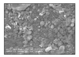
Fig. 3. Scanning Electron Microscopy (SEM) of Ag-PANI nanocomposite in concentration of  $0.1 \text{ M FeCl}_3$
