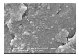
Fig. 2. Scanning Electron Microscopy (SEM) of Ag-PANI nanocomposite in concentration of 0.0125 M aniline
