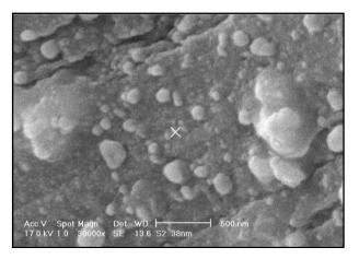
Fig. 1. Scanning Electron Microscopy(SEM) of Ag-PANI nanocomposite
