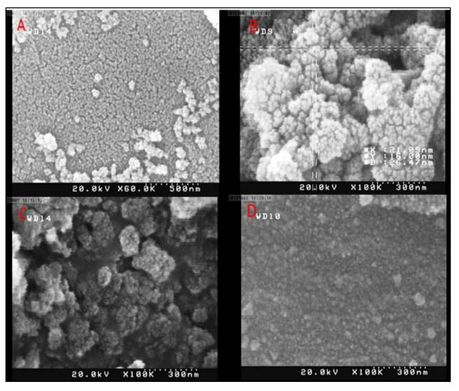
Fig. 2. SEM images of CuO/CuI nanocomposite at various reaction condition: A)at 80°C B) at 80°C in presence of oleic acid C) at 80°C low concentration D) at 120°C and low concentration.
