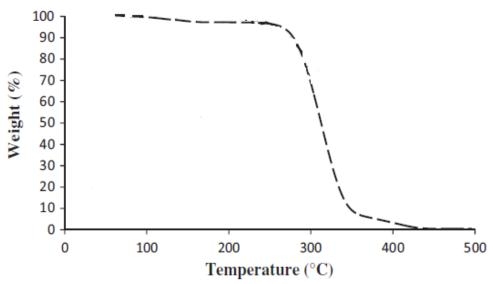
Fig. 3: TGA thermograms of nano-sized MIP.
