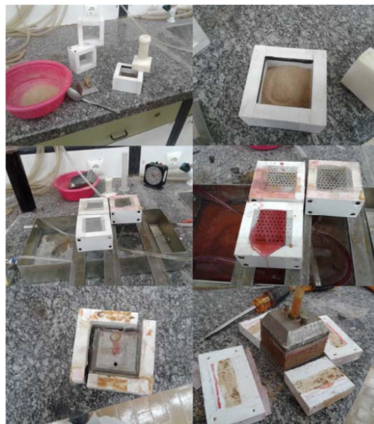
Fig. 12. Specimen preparing with the injection of colloidal Nano silica for direct shear test.
