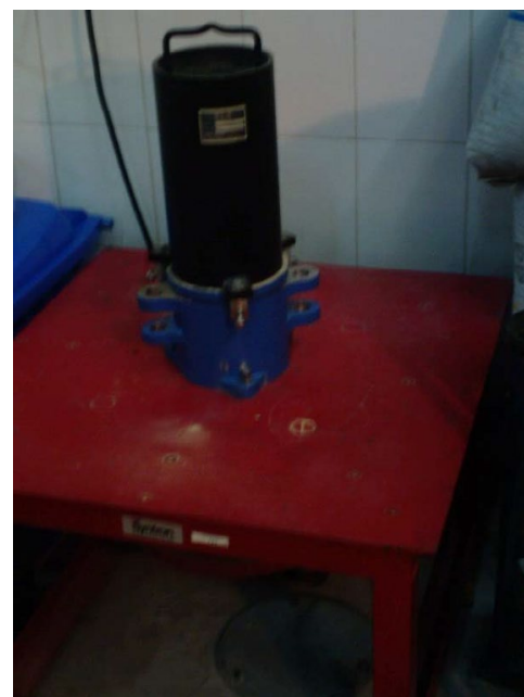
Fig. 5. Vibratory table apparatus in this study.
