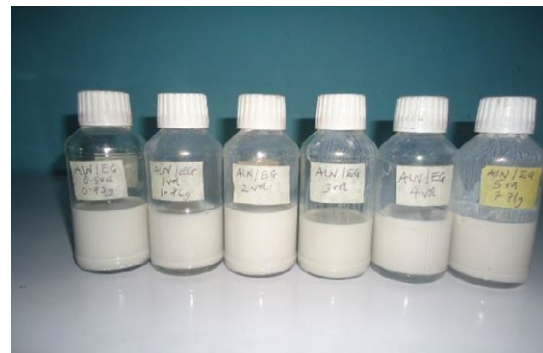
Fig. 2. Photographic image of just prepared AlN/EG nanofluids (0.5, 1, 2, 3, 4 and 5% vol. conc. from left to right).
