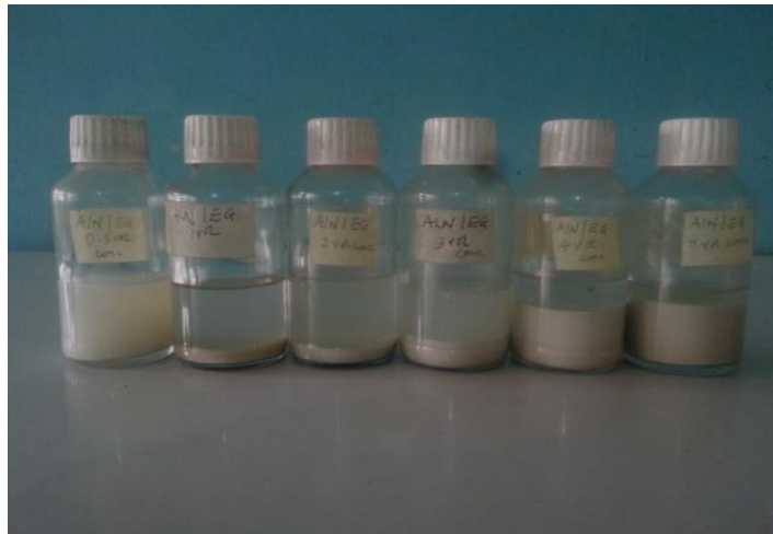
Fig. 7. Photographic image of dispersed AlN/EG nanofluids after six months (0.5, 1, 2, 3, 4 and 5 % vol. conc. from left to right).
