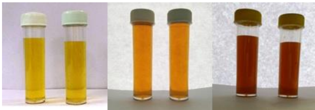
Fig. 2: The distinctive color of different sized silver Colloidal nanoparticles (a) yellow sol (b) darker yellow sol and (c) wine red sol.
