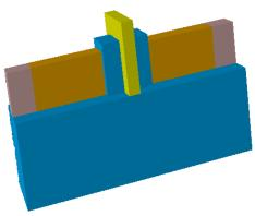
Fig. 2. Front view of proposed FinFET.
