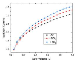
Fig. 8.  $log(I_{D})$  VS V<sub>GS</sub> curves for different gate materials.
