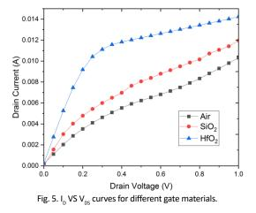
Fig.7. The dimension of gate in all the cases is kept same. From Fig.7, we can observe that the leakage current is same in both the cases [18-20], but Hafnium oxide resulted in higher ON current than silicondioxide and Air.
