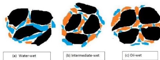
Fig. 6. Wettability alteration (a) Water-wet (b) Intermediate-wet (c) Oil-wet.
