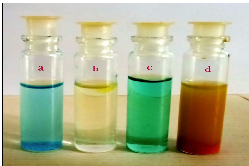
Fig. 1. Colour changes during the formation of RS-Cu 2 ONPs: a)- CuSO 4 Solution; b)- RS extract; c)- Mixture of CuSO 4 Solution and RS extract and d)-After heating at 80 °C for 1 hour (Reddish-Brown colour indicated the formation of copper nanoparticles).
