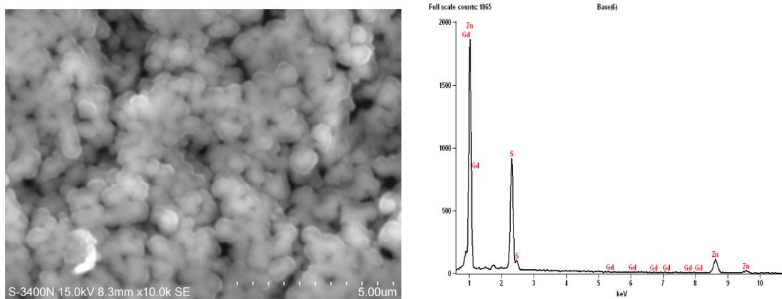
Fig. 2e. The SEM and EDAX spectrum of 5.5% Gd doped ZnS compound.
