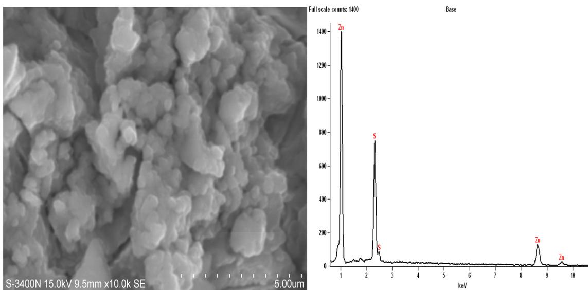
Fig. 2a. The SEM and EDA X spectrum of pure ZnS compound.
