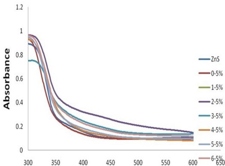
Fig. 4. The UV-visible spectrum of pure ZnS and Gd doped ZnS compounds with various concentrations.
