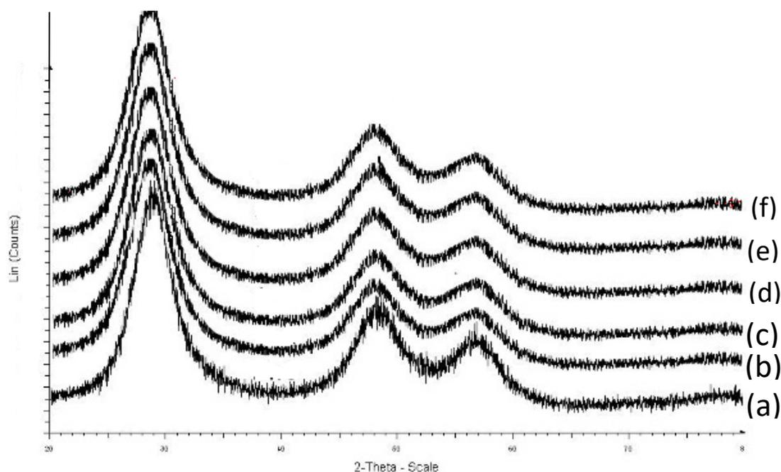
Fig. 1. X-ray diffraction (XRD) pattern of pure ZnS and Gadolinium doped ZnS nanoparticle samples (a) Pure ZnS (b) 0.5% Gd doped ZnS (c) 1.5% Gd doped ZnS (d) 2.5% Gd doped ZnS (e) 3.5% Gd doped ZnS (f) 4.5% Gd doped ZnS.
