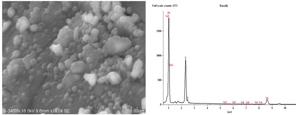
Fig. 2c. The SEM and spectrum of 3.5% Gd doped ZnS compound.
