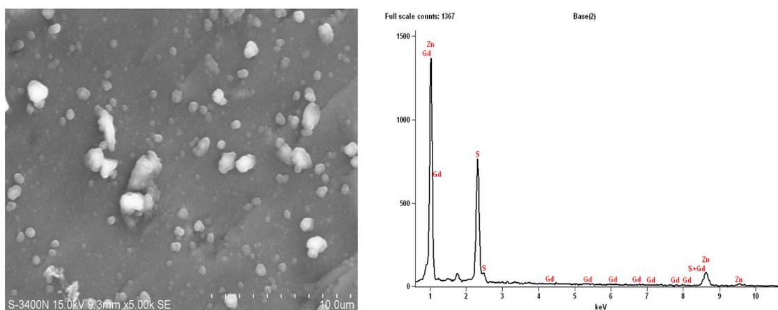
Fig. 2. b. The SEM and EDAX spectrum of 2.5% Gd doped ZnS compound.
